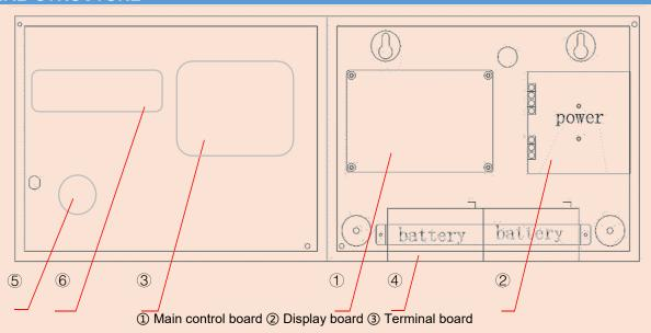
(4) AC/DC power module (5) Batteries (6)Buzz
